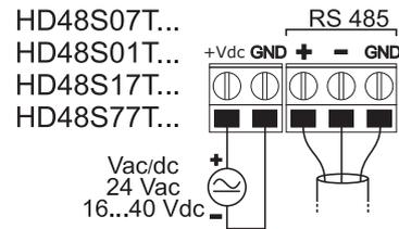
Thanks to RS485 output, several instruments can be connected to form a network. The instruments are connected in a sequence through a shielded cable with twisted pair for signals and a third wire for the mass.
